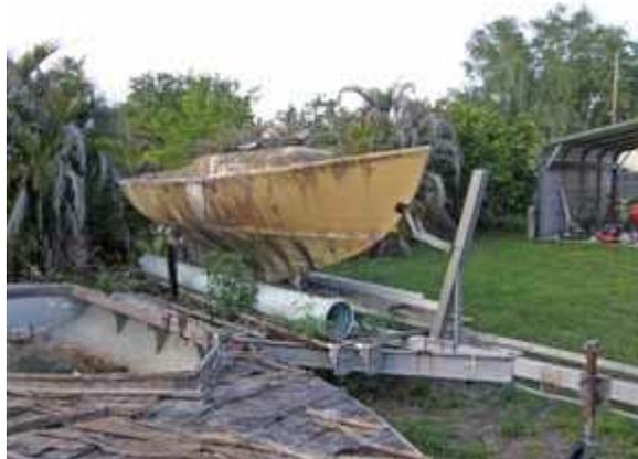
We jacked up the trailer, then removed the wheels and wheel bearings. We fixed the brakes with a Sawzall. We replaced all the wheel bearings and three of the four wheels and tires. One of the replaced wheels was still suitable as a spare. The Sawzall got another workout on a second powerboat trailer that dad found on a tree lawn and dragged home behind his station wagon. The cross-members were rotted, but the wishbone frame was sound. I had ideas of
